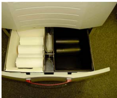
Waste drawer open showing empty cartridges and full waste bag.
