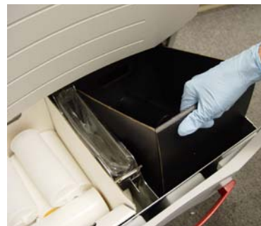
Removing model material waste bin liner for disposal.
