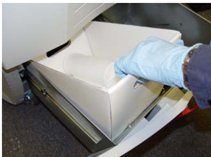
Removing support material waste bin liner for disposal.
