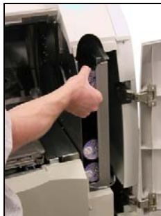
Insert cartridge flat side up, then lower into slot
