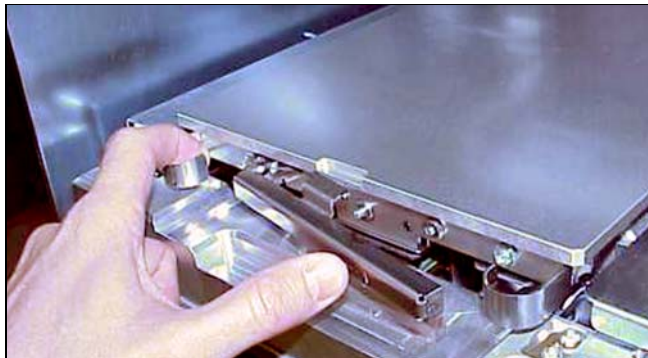
Unlatch platform and lift it out
