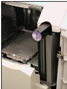
Insert cartridge flat side up, then lower into slot
