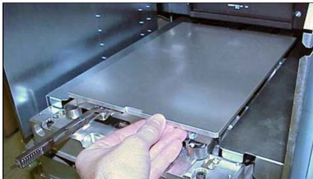
Install platform; verify latch
