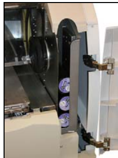
Insert cartridge flat side up, then lower into slot
