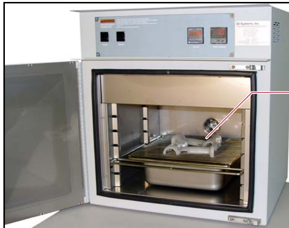
Dry finishing VisiJet parts on Finisher shelf
