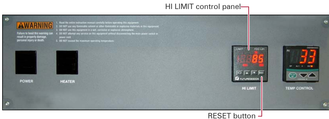
HI LIMIT panel with heater RESET button on the Finisher control panel
